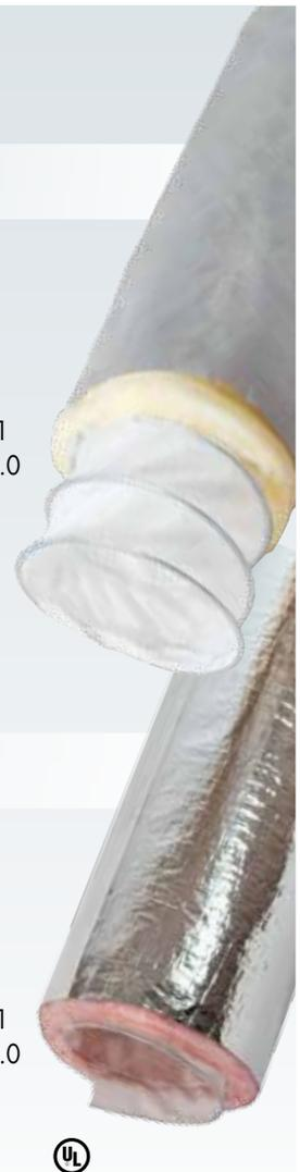
Flexmaster flexible ducting products are UL Approved as Class 1 Air Duct and have a Flame Spread Rating of not over 25 without evidence of continued progressive combustion and a Smoke Developed Rating of not over 50. Thermal resistance R4.2, R6 and R8.
